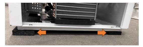
Alternatively, a hand truck or forklift can do the heavy lifting, but make sure the forks do not damage the condensing unit under the chamber. Also note that the center of gravity of the chamber may not be in the middle of the cabinet.
