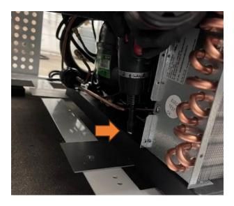
Step 4: **Having a second person to assist in this step can be helpful.** Using gloves, lift the condensing unit and slide out the unpainted metal supports (as shown in the photo below). Carefully lower the condensing unit to the ground, being careful not to damage the copper refrigerant lines. Make sure no part of the condensing unit is touching the chamber's frame. Save the unpainted metal supports just in case the chamber must be moved to a different location in the future.
