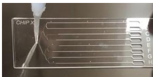
Figure 2: correct positioning of the tip for sample injection through the chip inlet
