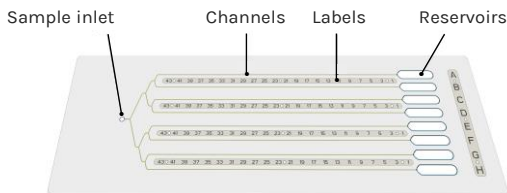
Figure 1: Schematic diagram showing the crystallization chip design
